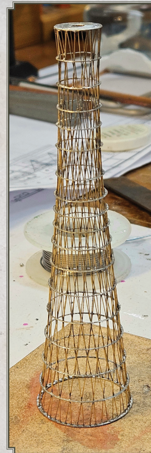
This sequence of images show the process of how the cage masts were constructed after a careful study of the ships plans. A jig was made to insure all the .020 brass rods would be correctly aligned with the center support and rings when soldered together.
