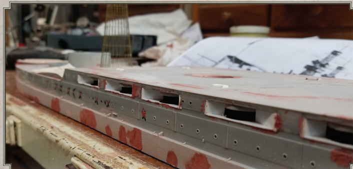
In-progress view of the 5-inch gun casemates which were lowered a full deck to match the 1916 configuration.
