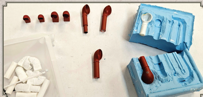
The surface fittings were modified and used as masters to create silicone molds.
