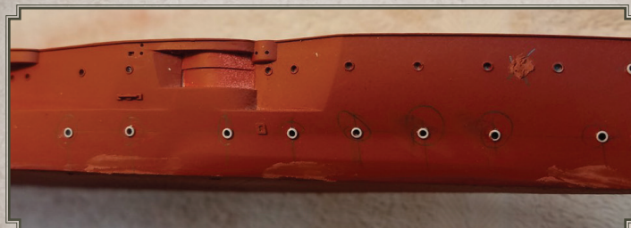
The new resin porthole frames were then glued to the hull.
