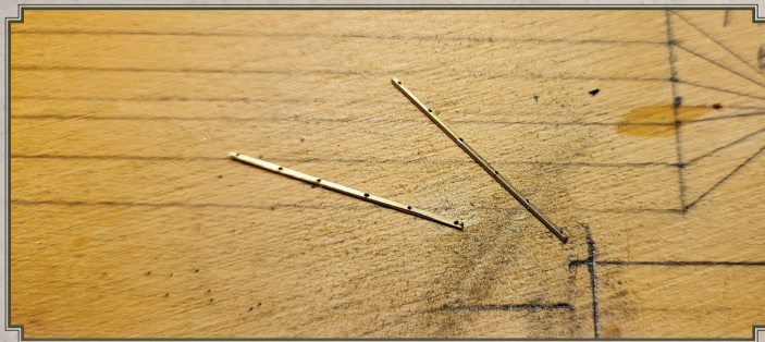
Detail view of the brass stock used to replicate the Arizona's antenna arrays.
