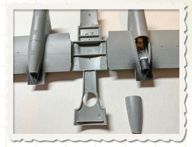
The two wing bottoms and fuselage underside molded as a single part. The main gear wells are trapped between the individual wing tops and bottom. The wing tops include the main engine nacelles. The cowling fronts are two parts and attach to the nacelles, leaving almost no join line. The engine exhausts are separate and are trapped by a rear nacelle top panel. The fit is incredible.
