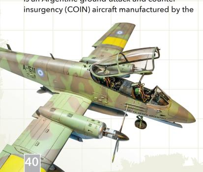
Armour plating protects the crew and engines from ground fire. The aircraft is powered by a pair of Turbomeca Astazou engines driving sets of three-bladed Ratier-Forest 23LF propellers that are also capable of being used as air brakes.
