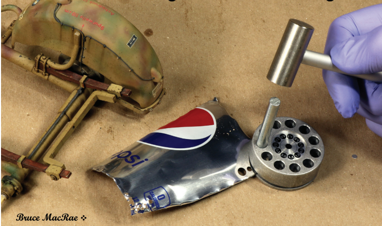
Making reflectors for the lights
